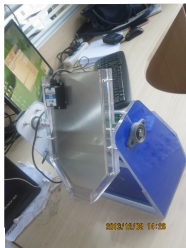
Figure 1. Sliding friction angle and rest angle measurement instrument.
